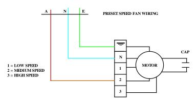
To alter the speed remove the active wire on the flex side from the terminal 2 and insert into terminal 1 for low speed or terminal 3 for high speed. Refer diagram below. Under no circumstances connect the neutral wire to terminals E, 1, 2 or 3.
