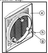
2. Put the Weather Cap Mounting Screws (p), into the holes within the collar section of the Weather Cap from the inside so the screws point out toward you. Slide on the rubber grommets (g) with the flat side up, then the white tabs (n), the washers (o) and hold them in place with the nuts (r) leave the nuts loose for now.
