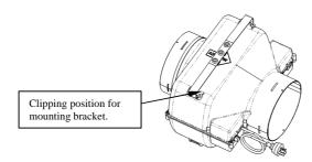
B). Utilise the four holes and four screws provided to fix the fan appropriately.
