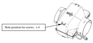
4. Plug fan into 240V AC power point.
