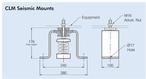
Load Nominal **Static Restraint Capacity Model Number** Defl. mm Horizontal, kN Vertical, kN Range, kg CLM-89 to 100 10-650 25 3.5 7.0
