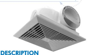
Airbox is a low profile, extraction fan that can be installed into tight ceiling spaces such as between floors or within cathedral ceilings. It features a non-return damper to eliminate backdraft and a high performance centrifugal impeller that produces powerful air flow and low noise. Models to suit 100mm and 150mm diameter duct sizes are available.
